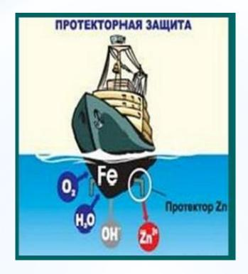
**Protector method:** a piece of a more active metal (protector) is attached to the protected metal structure, which serves as an anode and is destroyed in the presence of an electrolyte.
