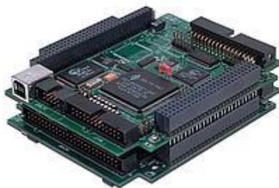
Рис. 4.33. PMAC2-PC/104 Motion Controller for 4 or 8 Axis фирмы Delta Tau Data
