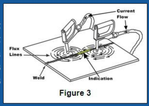
Because the magnetic field between the prods is travelling perpendicular to a line drawn between the prods, indications
