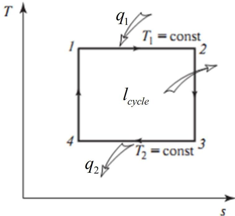
**Carnot cycle** is a reversible process in which: 1) heat exchange occurs at constant temperature; 2) transfer from one heat source to another occurs without heat exchange (adiabatically); 3) there is no friction in all the processes.
