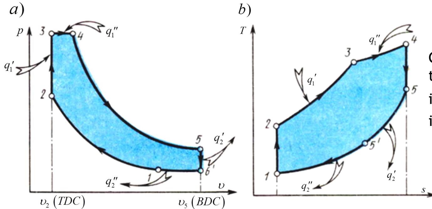
Generalized thermodynamic cycles in  $p$  $v$ -diagram (a) and in  $T$  $s$ -diagram (b)
