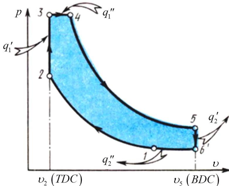
Any process in a cycle is characterized by one equation with two variables ( $p$ ,  $v$ ,  $T$  or  $s$ ), and the nodal point is determined by one parameter.
