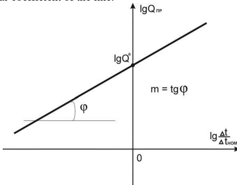
Pic. 2 Graph of dependence  $\lg Q_h$  on  $\lg \Delta t / \Delta t_{nom}$
