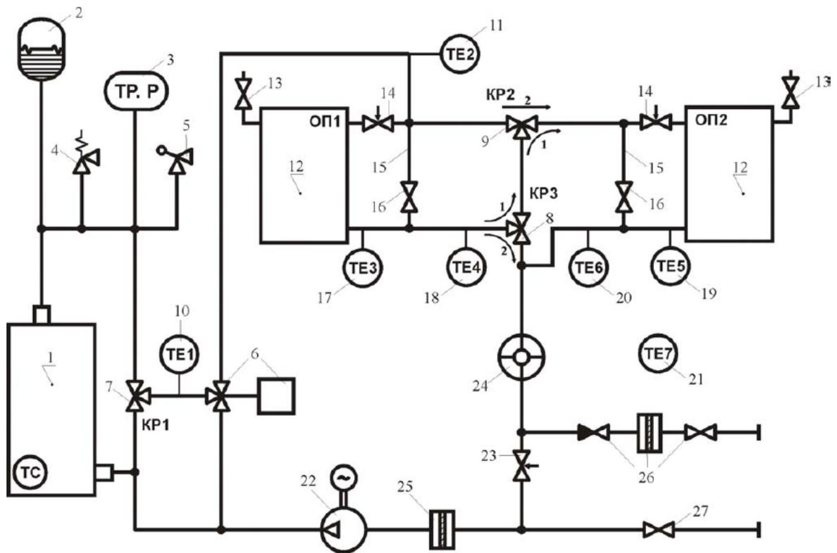
Fig.1. Hydraulic schematic diagram of the autonomous heating system.
