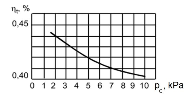
Dependence of efficiency of the Rankine cycle on the final pressure
