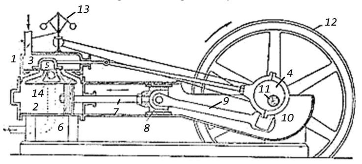
1 – slide box, 2 – cylinder, 3 – piston valve, 4 – eccentric,
