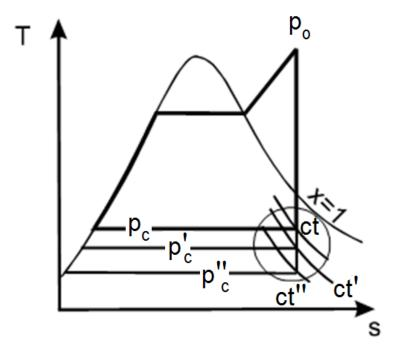
Rankine cycle at various final pressures (in Ts-diagram)
