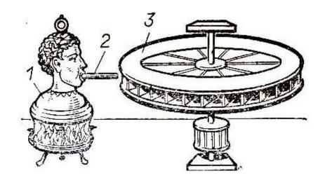
Scheme of conversion of heat energy into mechanical energy in turbine
