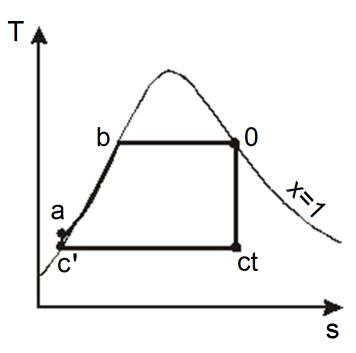
Rankine cycle with saturated steam in Ts-diagram
