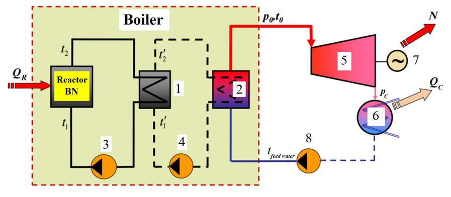
1 – heat exchanger; 2 – steam generator; 3 – main circulating pump 1;
