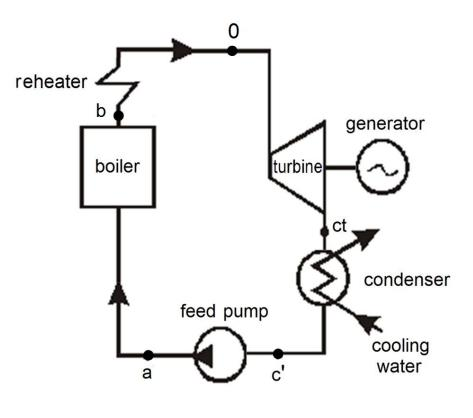
a-0 – isobaric heat supply to a working medium at initial pressure  $p_0 = const$
