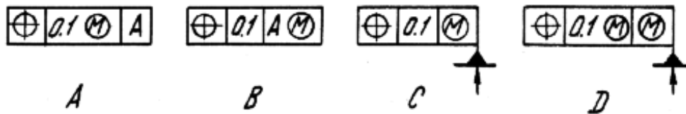
Fig. 6-10. Designation of dependent tolerances.
