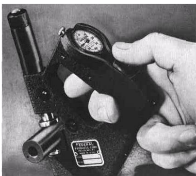
Fig. 4-4. Retractable contact snap gage.
