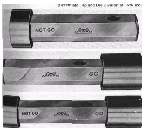
Fig. 5-6. Plain cylindrical plug gages. Top — single-end gages. Bottom — double-end gage.
