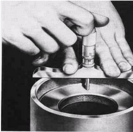
Fig. 12. Measuring depth of a shoulder with a depth micrometer.
