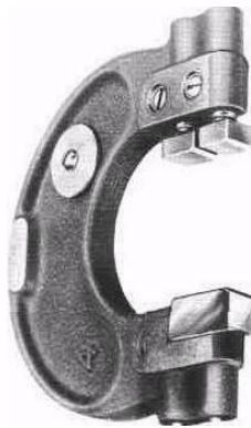
Fig. 2. Adjustable limits snap gage.
