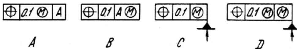
Fig. 10. Designation of dependent tolerances.
