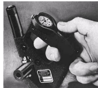
Fig. 7. Retractable contact snap gage.
