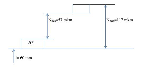
Tolerance zones of the coupled details limit gages.
