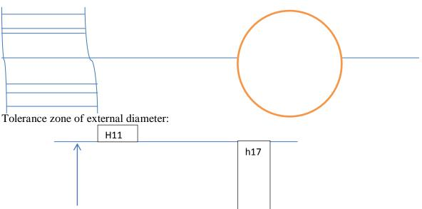
Tolerance zone of internal diameter:
