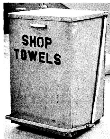
Fig. 12. Approved metal container for oily rags.
