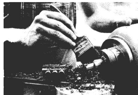
Fig. 8. Brushing is a safe way to remove chips.
