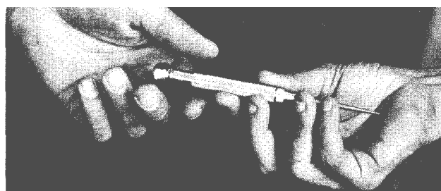
Fig. 11. A scribe is needle-sharp and hard enough to cut steel. If you are giving it to someone else, offer it handle first.
