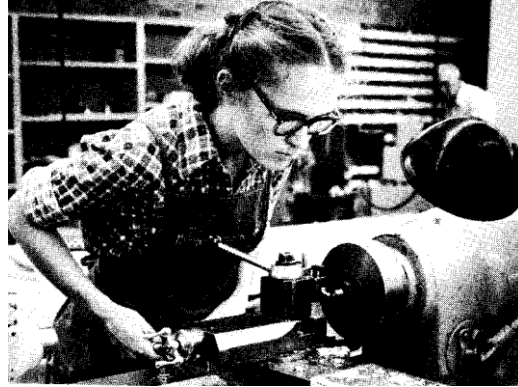
Fig. 2. Long, loose hair can get caught in machinery. Confine it in a cap or tie it back securely.
