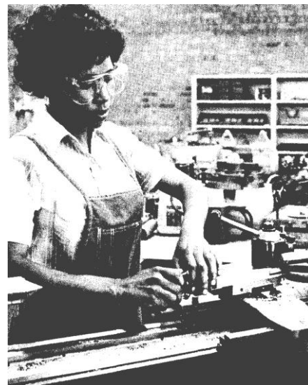
Fig. 4. Machine operator dressed properly for working safely at metal lathe or other machine tools.
