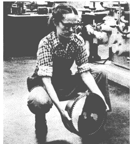
Fig. 9. There is a correct method for lifting heavy workpieces to the machine - lift heavy objects by using the strength in your legs, not your back.
