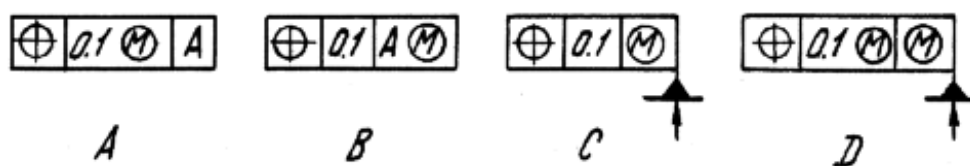
Fig. 10. Designation of dependent tolerances.
