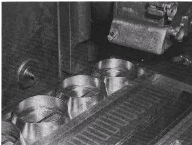
Fig. 22-11. Work mounted in V-blocks on magnetic chuck.
