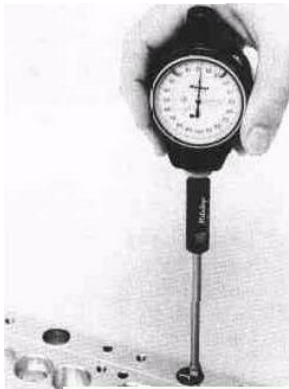
Fig.4-5. Dial indicating hole gage.
