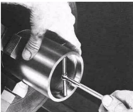
Fig. 2-10. Using a telescoping gage.
