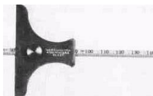
Fig. 2-2. Rule depth gage.
