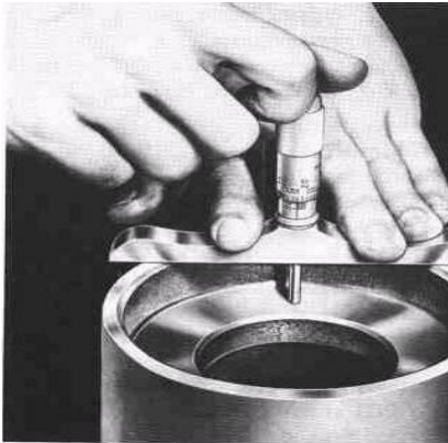
Fig. 3-4. Measuring depth of a shoulder with a depth micrometer.
