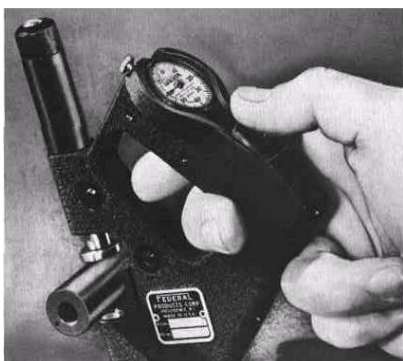
Fig. 4-4. Retractable contact snap gage.
