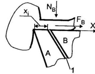
$$\sigma_N(x) = \frac{1}{b_1} \frac{dN_B}{dx}; \quad \tau_F(x) = \frac{1}{b_1} \frac{dF_B}{dx}.$$
