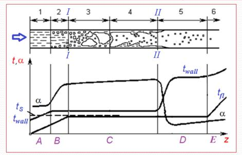
Here  $\alpha$  – heat transfer coefficient, W/(m<sup>2</sup>· °C);  $t_S$  – saturation temperature, °C;  $t_{wall}$  – wall temperature, °C;  $t_w$  – water temperature, °C
