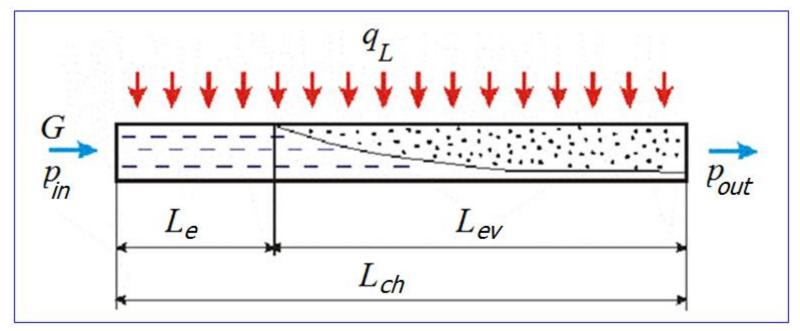
Here  $q_L$  - linear heat flux, W/m;  $L_{ch}$  - channel length, m;  $L_e$ ,  $L_{ev}$  - length of economizing and evaporation zones, m;  $p_{in}$ ,  $p_{out}$  - pressure at the channel inlet and outlet
