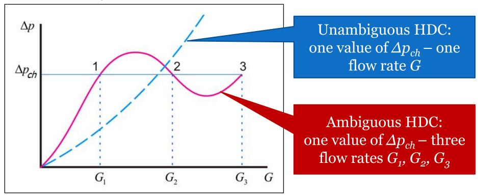
Here  $\Delta p_{ch} = p_{in} - p_{out}$  – pressure differential in the channel;  $p_{in}$ ,  $p_{out}$  – channel inlet and outlet pressures; G – mass flow rate
