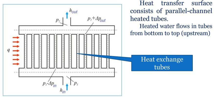
Here  $h_{in}$ ,  $h_{out}$  – water enthalpy at the inlet and outlet of heat transfer surface;  $\Delta p_{in}$ ,  $\Delta p_{out}$  – pressure drops at the inlet and outlet of tubes
