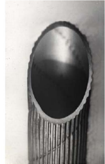
Fig 2. Tubes with longitudinal ribs
