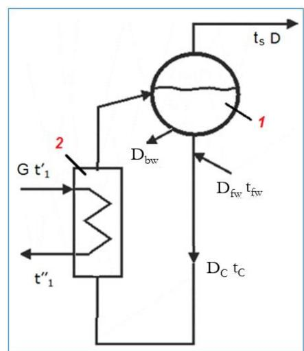
1 –separation volume 2 – economizer (E)-evaporator (Ev) D – steam flow rate  $D_{fw}$  – feedwater flow rate  $D_{C}$  – circulating water flow rate  $D_{bw}$  – blowdown water flow rate G – coolant flow rate
