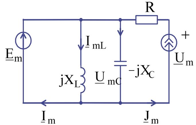
$$\underline{I}_{mL} = \frac{\underline{U}_{mC}}{jX_L} = 2e^{j0^\circ} \text{ A}$$
