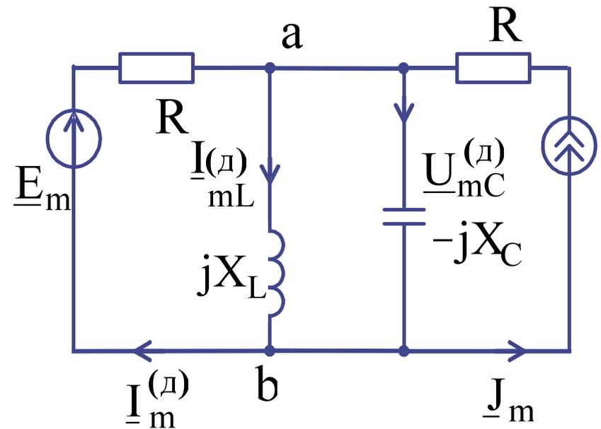
$$\underline{I}_{mL}^{(d)} = \frac{\underline{U}_{mC}^{(d)}}{jX_L} = \frac{282e^{j45^\circ}}{j100} =$$
