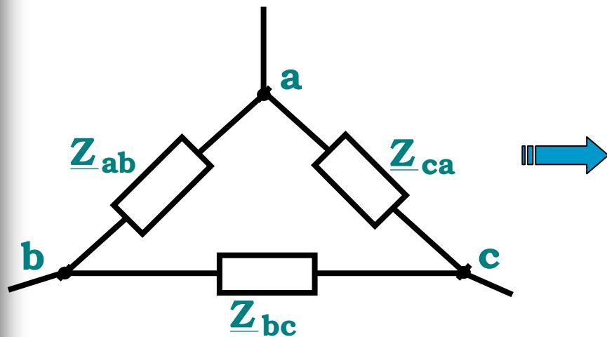
$$\underline{Z}_{ab} = \underline{Z}_a + \underline{Z}_b + \frac{\underline{Z}_a \underline{Z}_b}{\underline{Z}_c}$$
