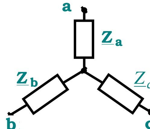
$$\underline{Z}_a = \frac{\underline{Z}_{ab} \underline{Z}_{ca}}{\underline{Z}_{ab} + \underline{Z}_{bc} + \underline{Z}_{ca}}$$
