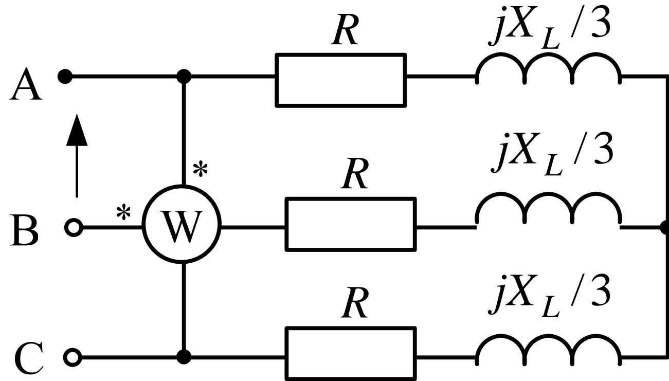
$$\underline{I}_A = \frac{\underline{E}_A}{Z} = \frac{\underline{E}_A}{R + \frac{jX_L}{3}}$$
