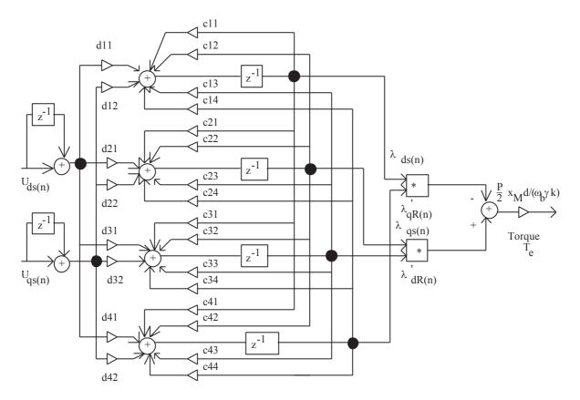
Fig.5.1. Complete discrete single-phase induction machine model based on bilinear transformation method (Tustin)
