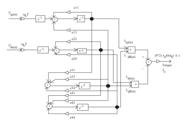
Fig.5.2. Complete discrete single-phase induction machine model based on forward-difference method (Euler)
