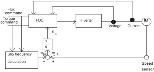
Fig. 1.4. Indirect vector control method
