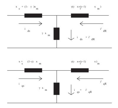
Fig. 3.7. Flux linkage equivalent circuit with arbitrary turn ratio
