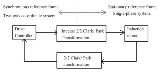
Fig. 3.11. Block diagram of transformation of frames and co-ordinate systems for single-phase induction motor vector control
