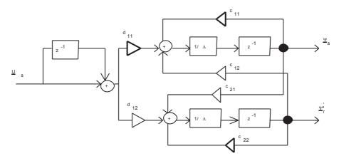
Fig. 4.1. The induction machine discrete model
