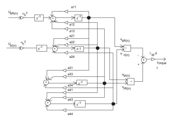
Fig. 4.3. Complete discrete induction machine model based on forward-differences method (Euler)
