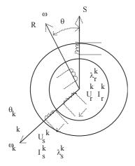
Fig. 2.4.Model of the three-phase induction machine with fictive one stator winding and one rotor winding (space vector notations) represented in a common arbitrary reference frame
