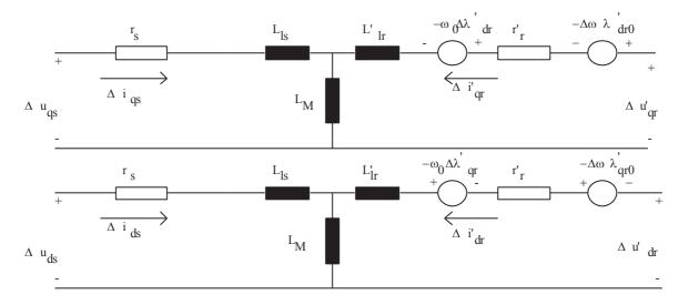
Fig. 6.1. Small-signal stationary reference-frame equivalent circuits for a three-phase, symmetrical induction machine
