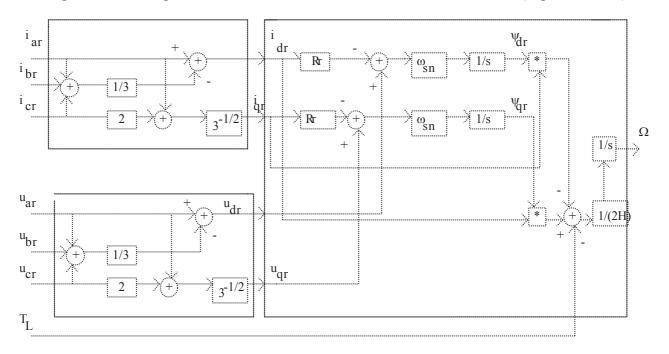
Fig. 2.9. Block diagram of the induction machine in rotor reference frame (wound rotor case)
