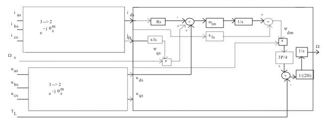
Fig. 2.15. Block diagram of the induction machine in synchronous reference frame (linked to magnetising current space vector)
