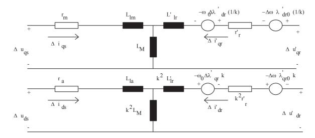
Fig. 6.2. Small-signal stationary reference-frame equivalent circuits for a single-phase, unsymmetrical induction machine
