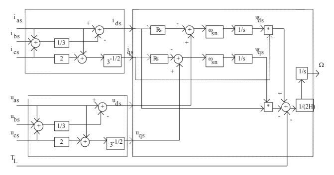
Fig. 2.7. Block diagram of the induction machine in stationary reference frame
