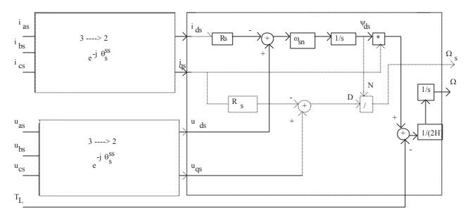
Fig. 2.10. Block diagram of the induction machine in synchronous reference frame (linked to stator flux)
