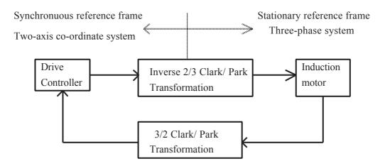
Fig. 2.18. Block diagram of transformation of frames and co-ordinate systems for induction motor vector control
