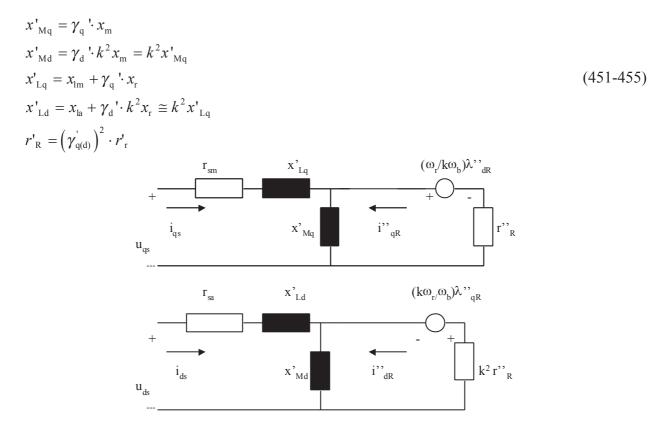
Fig.3.9. Equivalent linear d-q inverse  $\Gamma$  form circuit for the unsymmetrical single-phase induction machine
