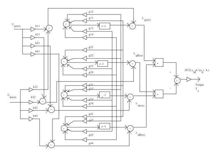
Fig. 5.3. Complete discrete single-phase induction machine model based on backward-difference method
