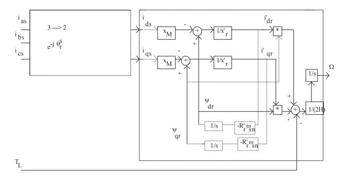
Fig.2.8. Block diagram of the induction machine in rotor reference frame (cage rotor case)
