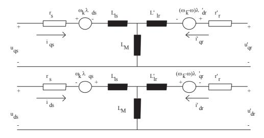
Fig. 2.17. Arbitrary reference-frame equivalent circuits for a three-phase, symmetrical induction machine
