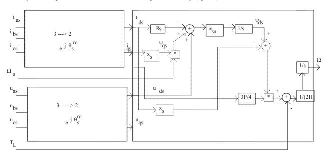
Fig. 2.14. Block diagram of the induction machine in synchronous reference frame (linked to rotor current space vector)
