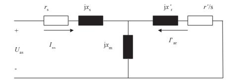
Fig. 3.3. Equivalent circuit of the symmetrical single-phase induction machine for the steady-state operation analysis
