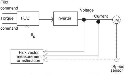
Fig. 1.5. Direct vector control method
