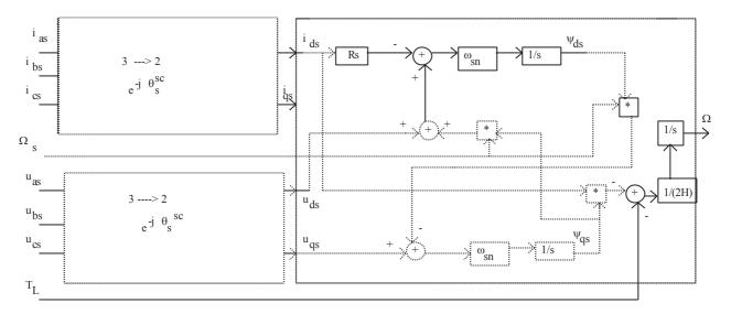
Fig. 2.13. Block diagram of the induction machine in synchronous reference frame (linked to stator current space vector)
