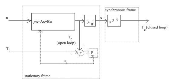
Fig. 2.16. Block diagram form of the induction machine mathematical model
