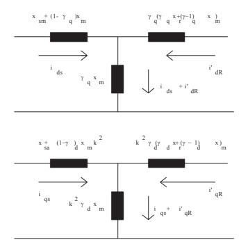
Fig. 3.10. Flux linkage equivalent circuit with arbitrary turn ratio for unsymmetrical single-phase induction machine
