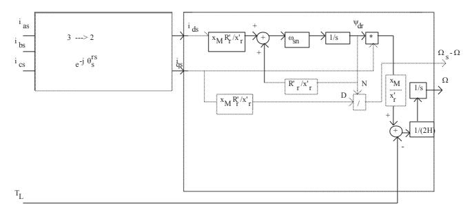
Fig. 2.11. Block diagram of the induction machine in synchronous reference frame (linked to rotor flux)
