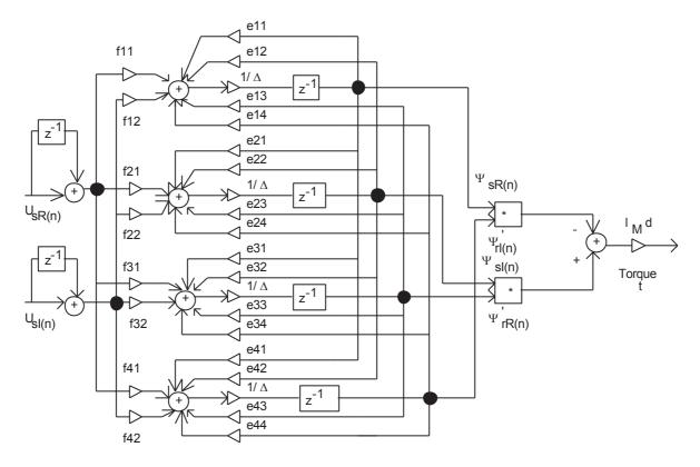
Fig. 4.2. Complete discrete induction machine model based on bilinear transformation method (Tustin)
