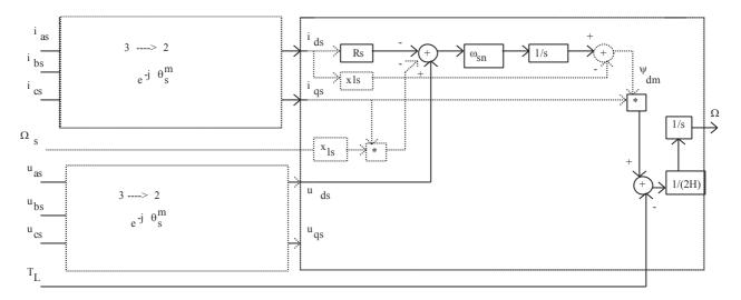
Fig. 2.12. Block diagram of the induction machine in synchronous reference frame (linked to air-gap flux)
