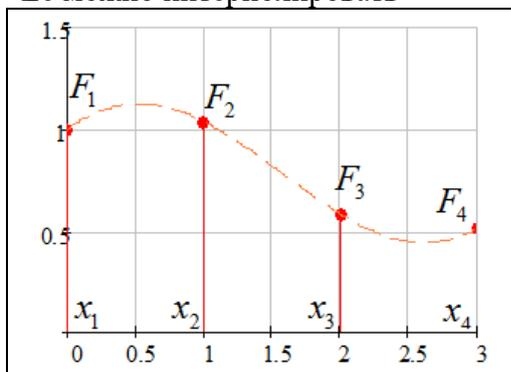
$$F(x) = \frac{L_1(x)}{L_1(x_1)} F_1 + \frac{L_2(x)}{L_2(x_2)} F_2 + \frac{L_3(x)}{L_3(x_3)} F_3 + \frac{L_4(x)}{L_4(x_4)} F_4$$
