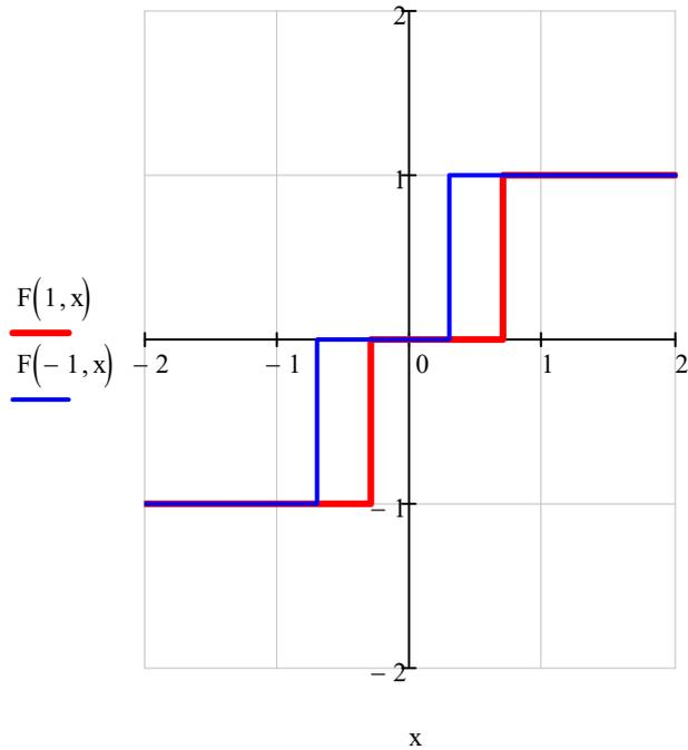
$$F(v, x) := \text{if}(v > 0, F(x - q), F(x + q)) \quad k_1 := 0.4 \quad T_1 := 1.5 \quad D(t, x) := \left( \begin{array}{c} x_1 \\ \frac{-x_1}{T_1} - \frac{k_1}{T_1} \cdot F(x_1, x_0) \end{array} \right)$$
