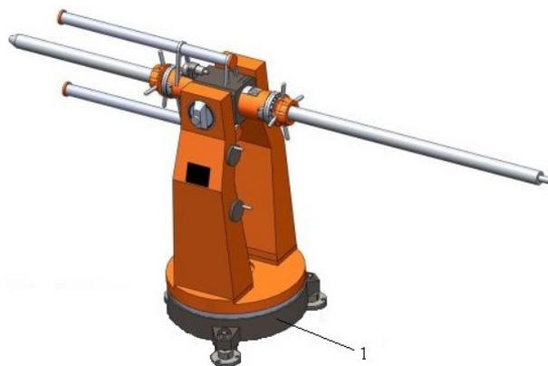
Fig. 1. Pan and tilt rotary system UNP-3
