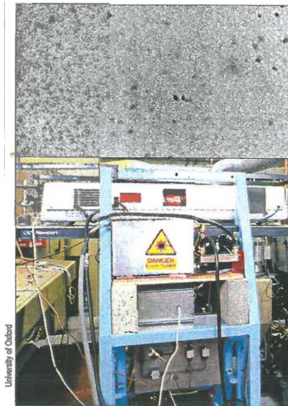
Below: copper vapour laser helps to optimize coatings deposited by vacuum plasma spraying. Left: metallic particles of 63 to 90 μm in diameter inside a 15 000 °C plasma.
