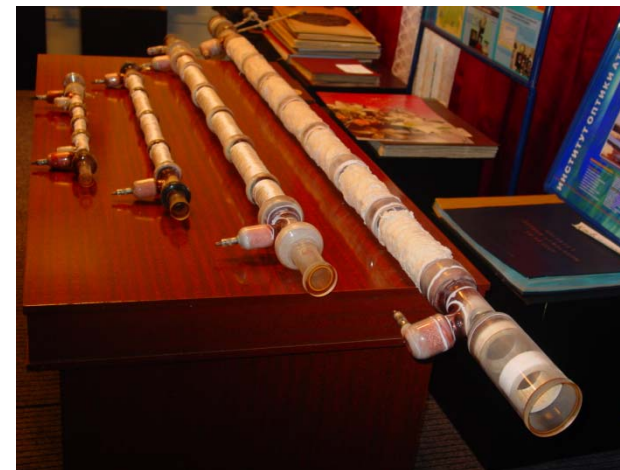
le vapor laser and one of the laser tube construction, Institute of Atmospheric optics SB RAS, Tomsk
