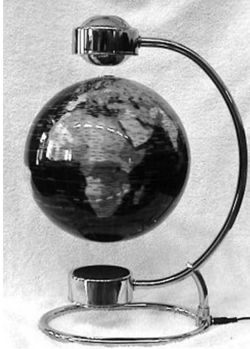
Fig. 14.21 Floating globe using magnetic suspension with feedback.
