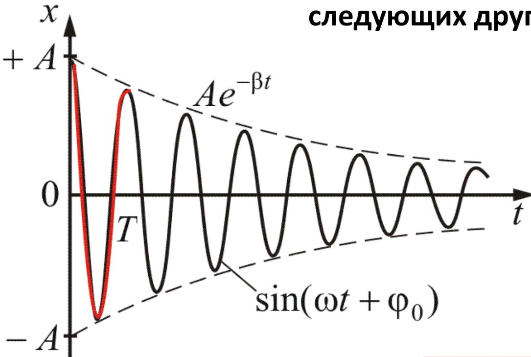
$$\begin{aligned}\frac{A(t)}{A(t+T)} &= \frac{A_0 e^{-\beta t}}{A_0 e^{-\beta(t+T)}} = \\ &= \frac{e^{-\beta t}}{e^{-\beta t} e^{-\beta T}} = e^{\beta T}\end{aligned}$$
