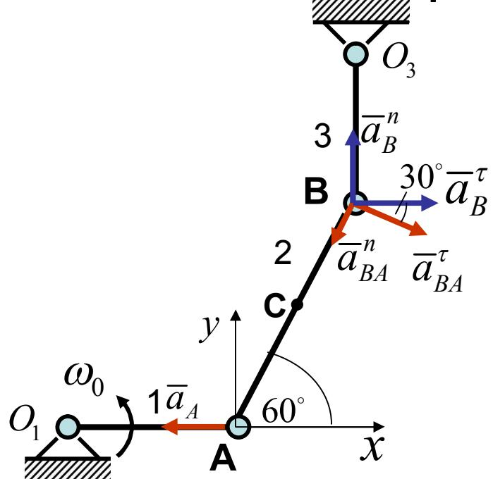
$$a_A = \bar{a}_A^n = \omega_0^2 O_1 A = \omega_0^2 r;$$
