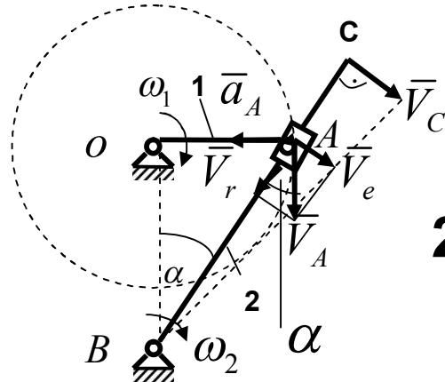
$$1. \quad V_A = \omega r; \quad a_A = a_A^n = \omega^2 r.$$
