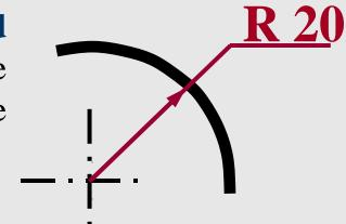
The radius dimension line is placed on that representation where the arc is projected in true shape.
