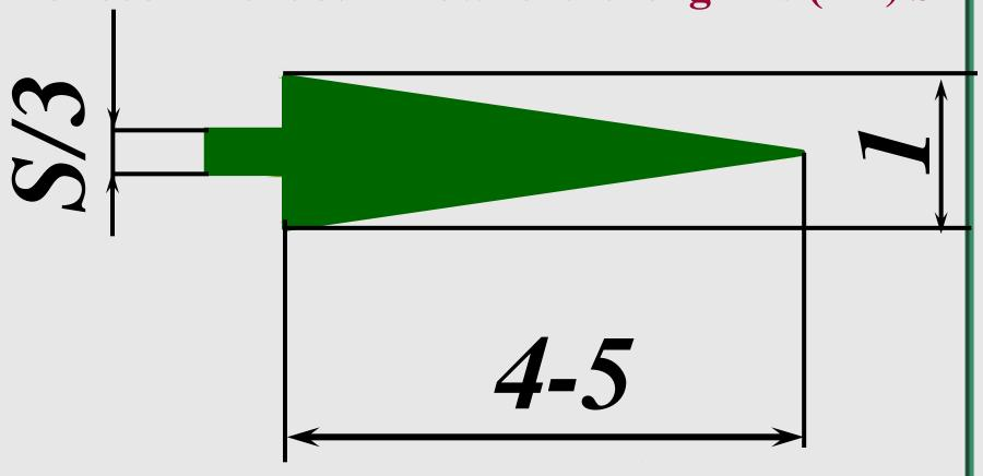
The length of arrowheads should be approximately equal for all dimensions of a given drawing.
