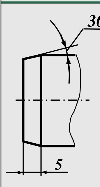
At any other value of the angle two dimensions are printed - a linear one and an angle ones.
