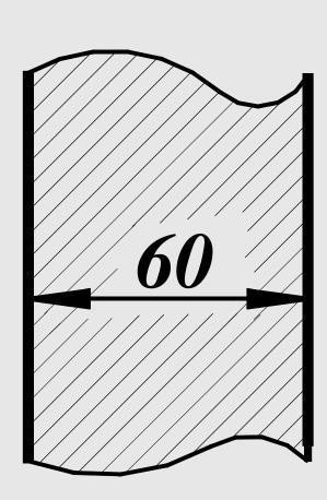
If it is necessary to print a dimension figure on an axis line or in a hatched section, the axis/hatching line may be broken.
