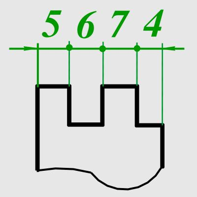
When printing a group of adjacent small dimensions, replace the arrowheads by clearly **printed dots or hatching lines on the extension lines**
