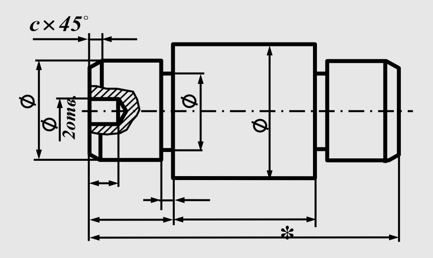
Dimensions of chamfers and grooves are not included in a dimension chain
