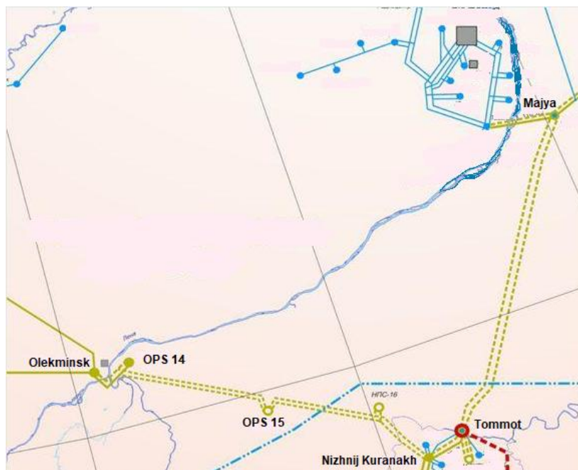
Figure 1.8 – Sketch map of 220 kV transmission lines: OPS – oil pumping station
