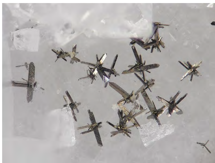
Fig. 47. Trillings of prismatic crystals of arsenopyrite (Clara Mine, Oberwolfach, Wolfach, Ortenaukreis, Freiburg Region, Baden-Württemberg, Germany)
