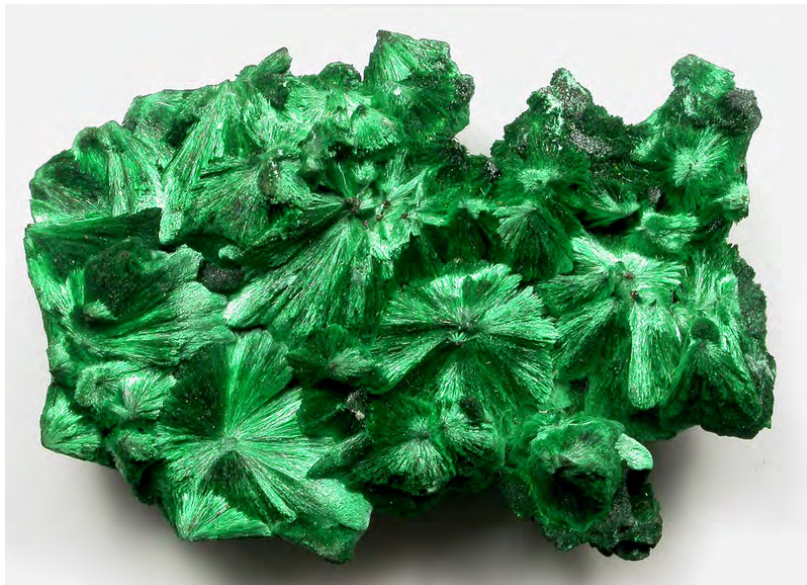
Fig. 84. Radial-radiant structure of malachite aggregates (Mashamba West Mine, Sicomines copper-cobalt project, Kolwezi mining district, Lualaba, DR Congo)
