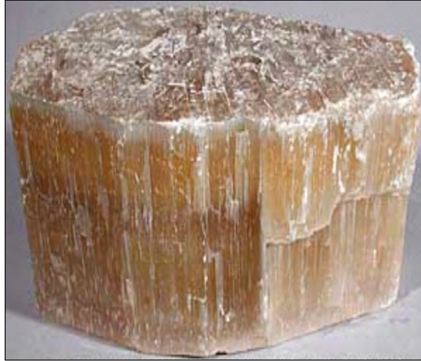
Fig. 24. Parallel-columnar intergrowth of fine-fiber crystals of gypsum with a silky sheen (selenite), as example of "grooved vein"
