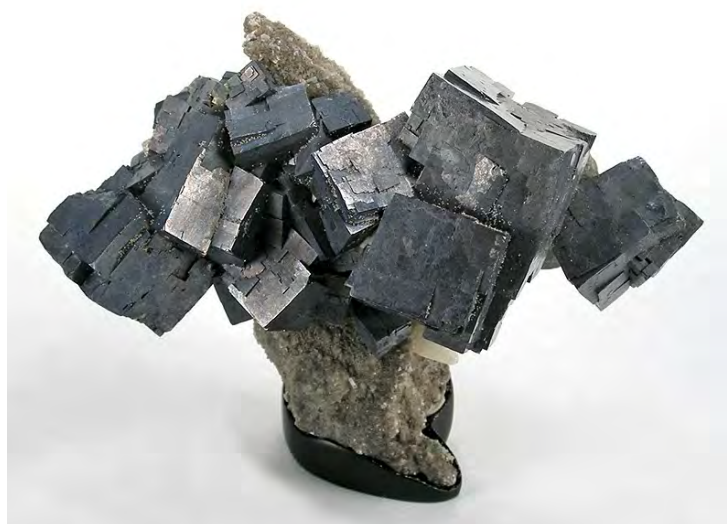
Fig. 41. Cubic crystals of galena with a characteristic cleavage at an angle of 90° (Sweetwater Mine, Ellington, Reynolds County, Missouri, USA)
