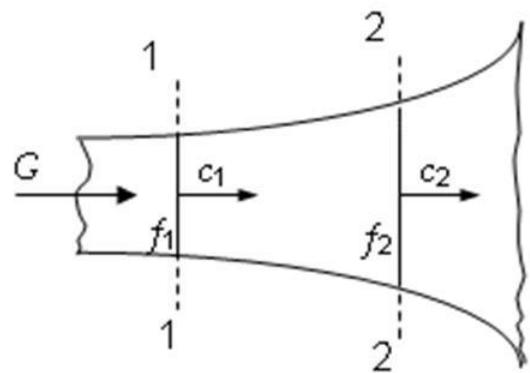
$$\begin{aligned} G &= \frac{M}{\tau} = |\tau - \text{время пребывания}| = \\ &= \frac{\rho V}{\tau} = \frac{\rho f x}{\tau} = \left| \frac{x}{\tau} \right| = c = \rho f c \\ G &= f_1 c_1 \rho_1 = f_1 c_1 / v_1 = f_2 c_2 / v_2 = \text{const} \end{aligned}$$
