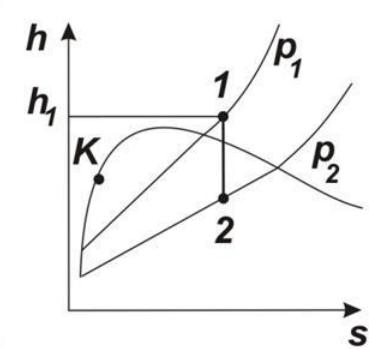
$$c_2 = \sqrt{2(h_1 - h_2) + c_1^2} = \sqrt{2(h_0 - h_2)}$$
