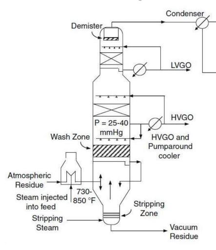
The distillate is withdrawn as light vacuum gasoil and two other cuts, medium vacuum gasoil and heavy vacuum gasoil.
