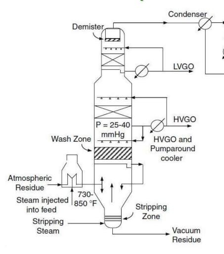
To minimize thermal cracking and coking, steam is injected in the heater tube passes.
