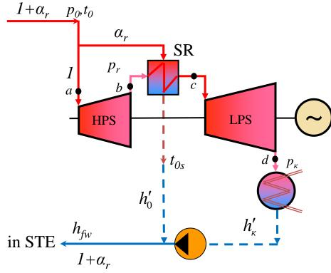
$$H_{i} = (h_{0} - h_{nn}^{*}) + (h_{nn} - h_{\kappa}) = H_{i}^{YBJ} + H_{i}^{YHJ};$$
