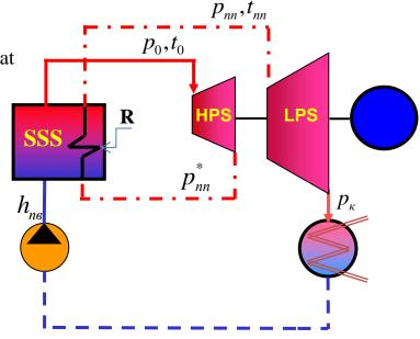
$h_0$  is enthalpy of the starting point of steam expansion in the turbine,  $= f(p_0, t_0)$   $h_{nnt}^*$  is enthalpy at the end of theoretical steam expansion in HPS,  $= f(p_{nn}^*, s_0)$
