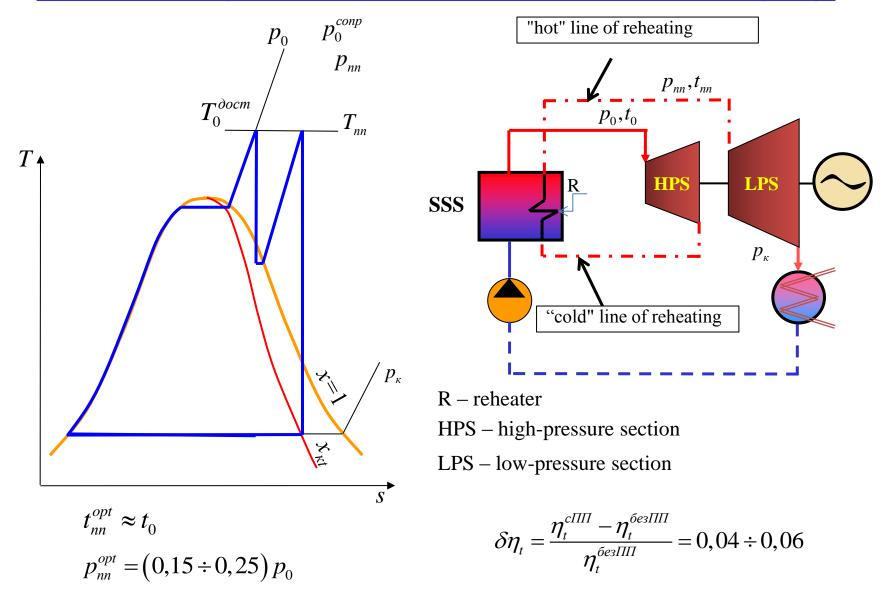
The schematic diagram shows the so-called **fired** steam reheating
