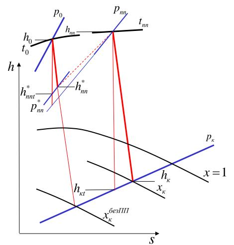
$h_{nn}$  is is enthalpy of the starting point of steam expansion in LPS,  $=f(p_{nn}, t_{nn})$
