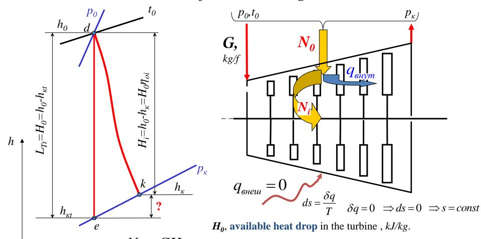
$N_0 = GH_0$ , available power (power of an ideal turbine), kW.  $H_i$ , real heat drop in the turbine, kJ/kg.
