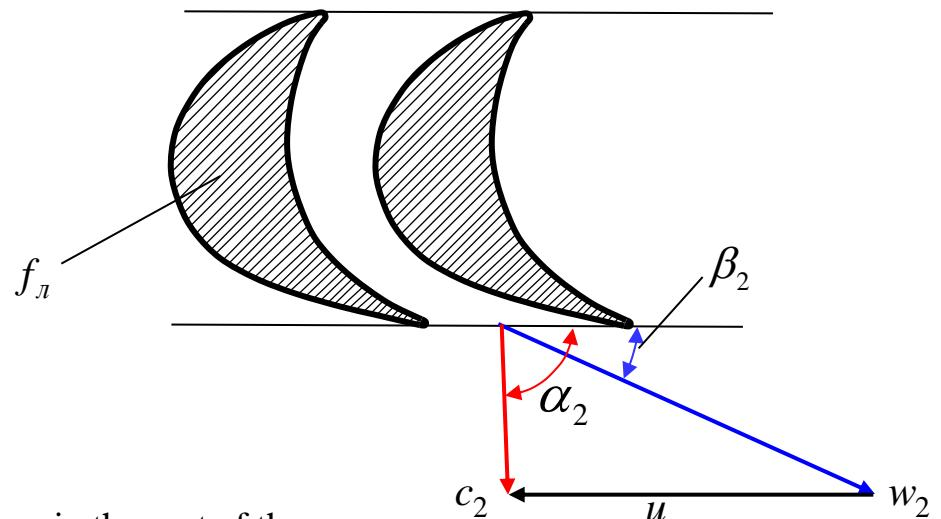
Determine the tensile stress from centrifugal forces in the root of the blade with constant section:
