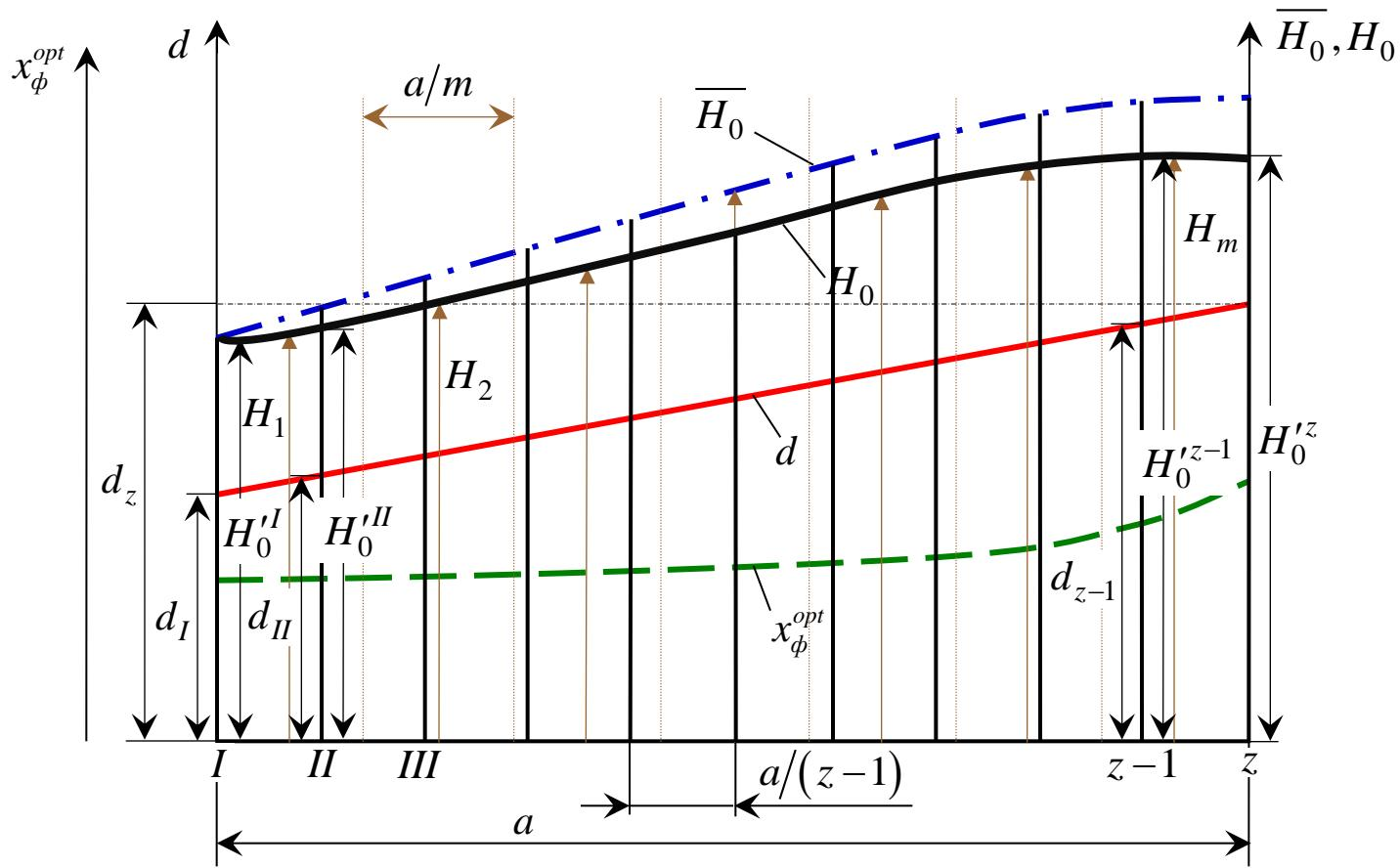
7. Determin the diameter and available heat drop of each of the  $z$  stages
