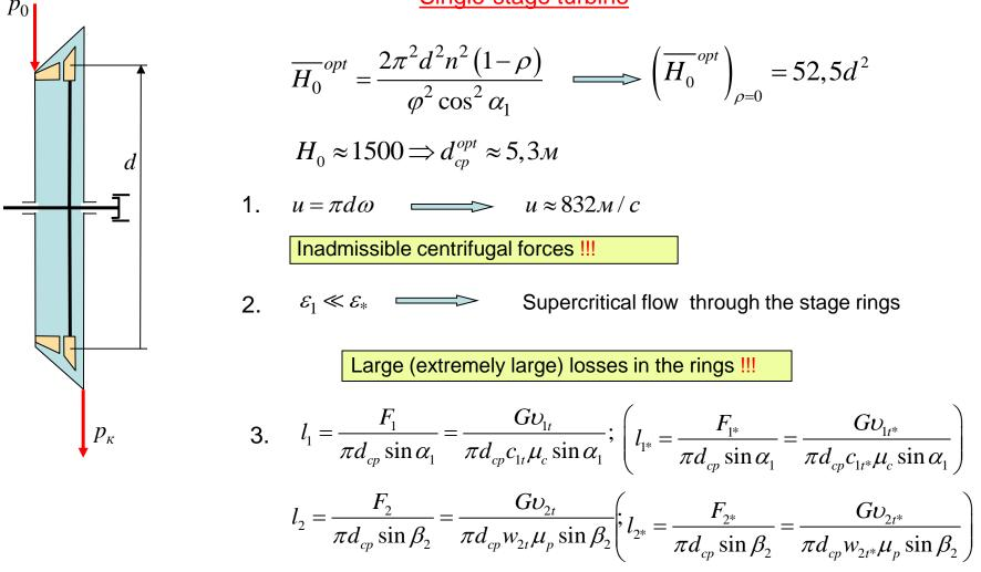
**Conclusion:** Single-stage turbine either cannot be designed to implement currently implemented heat drops (claim 1); or (in case of advanced materials) it is uneconomical and exigeant.
