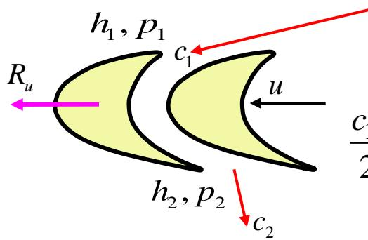
$$\frac{c_1^2}{2} + h_1 = \frac{c_2^2}{2} + h_2 + L_u$$
