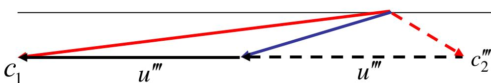
**Third dogmata:** EF will be of the highest level if the exit angle of the absolute velocity from rotor blades is  $90^\circ$ , i.e., the flow direction is parallel to the rotation axis
