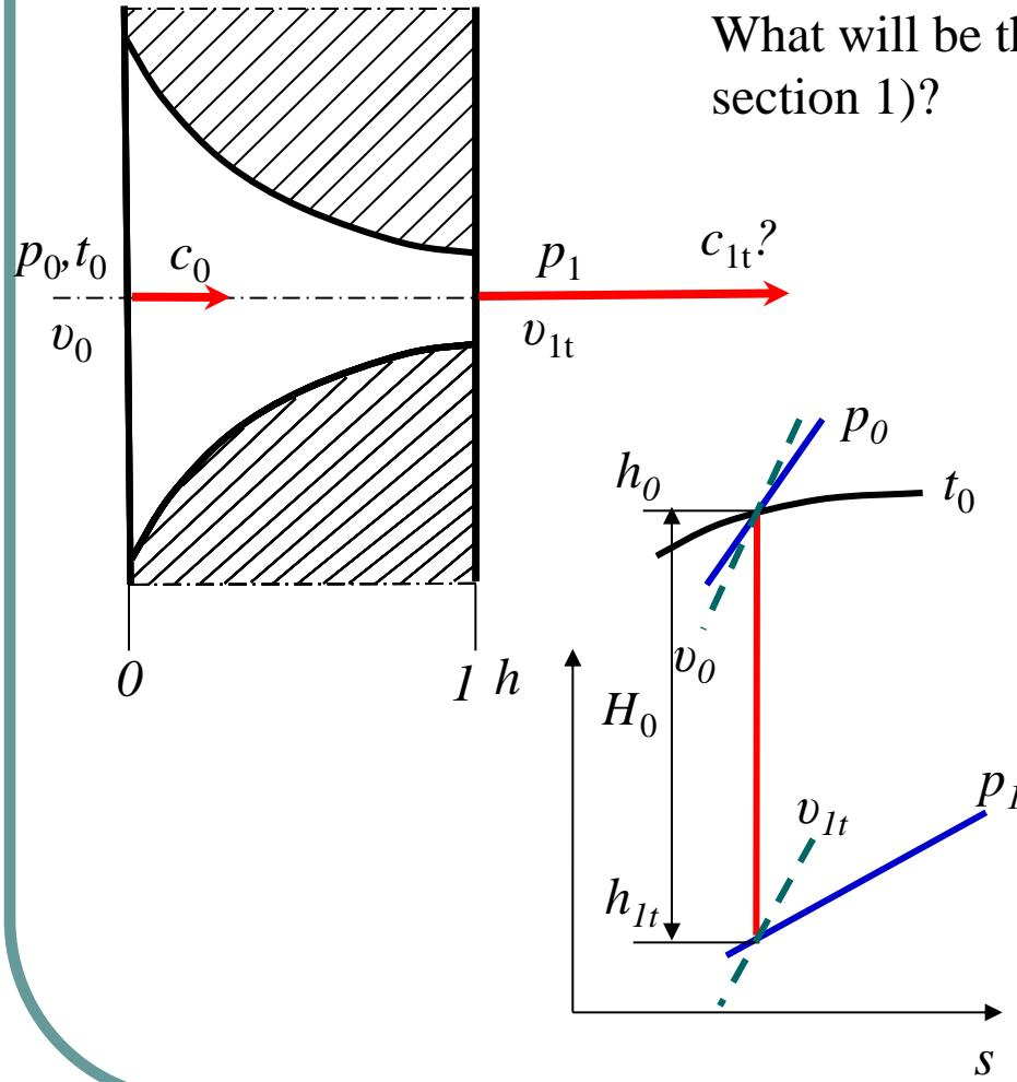
What will be the flow rate at the channel outlet (in section 1)?
