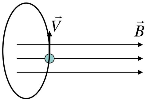
$$\vec{V} \perp \vec{B} \quad (\alpha = 90^\circ)$$
