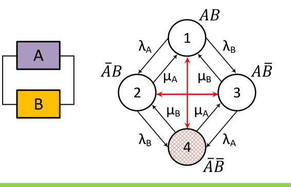
Since the components in the <u>second case</u> are statistically identical, it is irrelevant which item fails first – <u>the consequences</u> for the system <u>are the same</u>.
