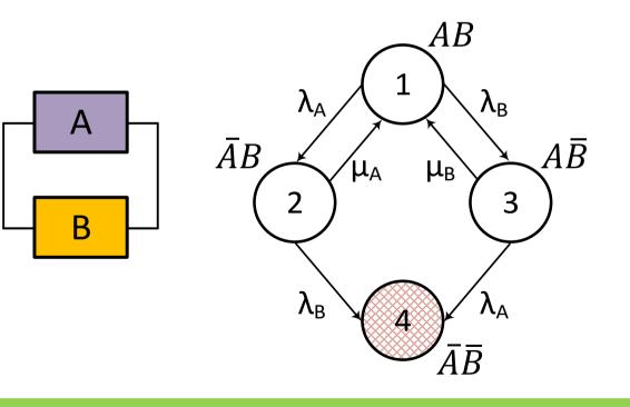
Finally, failed components from state 4 may be repaired, returning the system into states 2 or 3.
