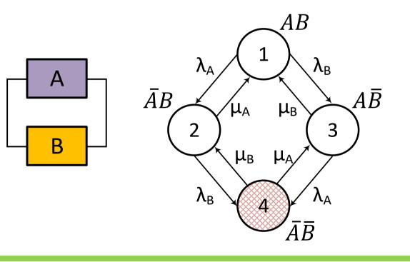
Note that each arc corresponds to a <u>single failure/repair event</u> – no two events can occur simultaneously!
