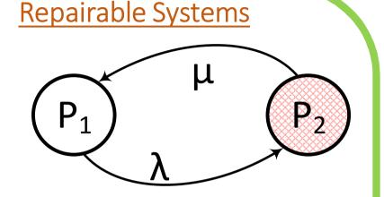
On the right side we have <u>as many terms as the number of arcs</u> adjacent to a current state. Each arc is represented by its rate times the probability of the originate state.
