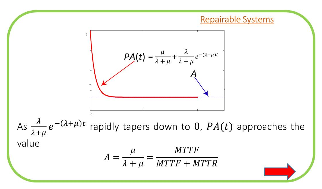
Since usually  $\mu \gg \lambda$ , PA(t) reaches its steady-state value very fast. So, instead of solving differential equations, we can obtain a steady-state solution a lot easier.
