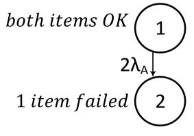
However, only one failed item is under repair in state 2, so the rate of reverse transition is still  $\mu_A$ .
