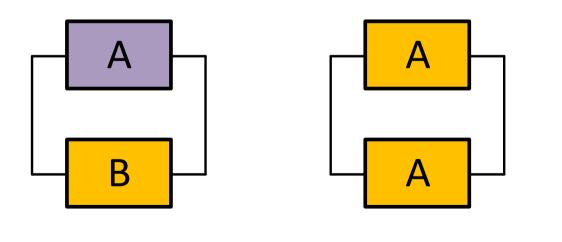
Starting from the initial state 1 in <u>the first case</u>, two events may happen: <u>either</u> component A or component B may fail (states 2 and 3). Those events are not the critical ones – <u>the system is still</u> in operable state.
