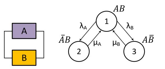
Components still operating in states 2 and 3 may fail as well, thus causing system failure (state 4).
