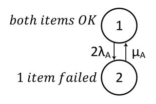
State 2 still has one operable component that may fail, resulting in system failure.
