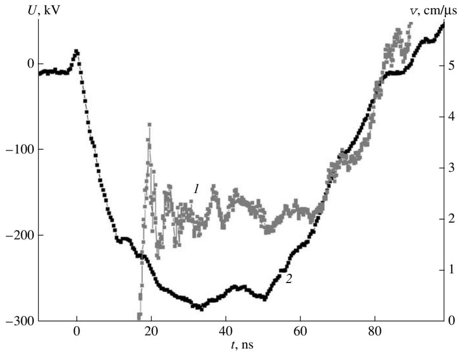
**Fig. 5.** Time-dependent expansion velocity of EE plasma in a diode with a 60-mm-diameter carbon-fabric cathode calculated from formula (2) at gaps of 10.5–13.5 mm (curve 1). Curve 2 is the applied voltage.
