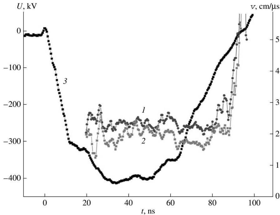
**Fig. 3.** Change in the EE-plasma expansion velocity during generation of an electron beam in a planar diode with a 45-mm-diameter carbon-fabric cathode at anode–cathode gaps of (1) 9.5 and (2) 15.0 mm. Curve 3 is the voltage applied to the diode.
