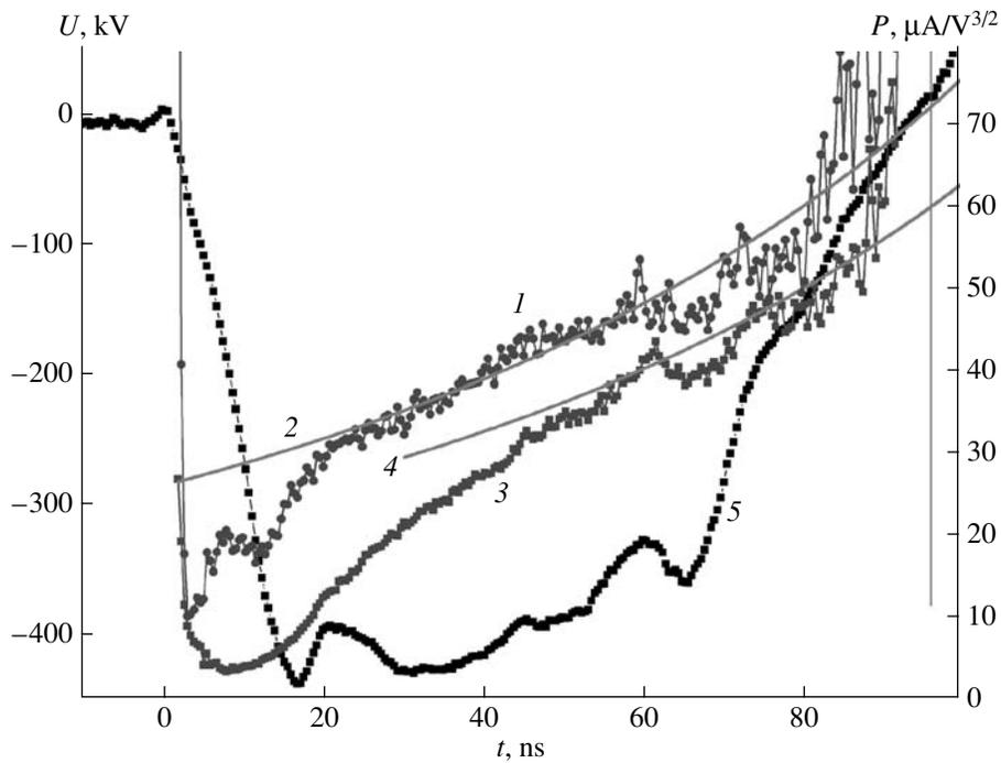
**Fig. 6.** (1, 3) Experimental and (2, 4) calculated values of the planar-diode perveance for (1, 2) multispike and (3, 4) solid copper cathodes at an anode–cathode gap of 12 mm. Curve 5 is the voltage applied to the diode with the copper cathode.
