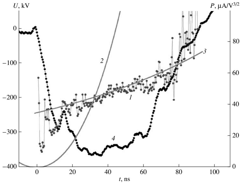
**Fig. 8.** (1) Experimental (dots) and (2, 3) calculated (from (4) and (3), respectively) values of the perveance of a planar diode with a multispike cathode at a gap of 12.5 mm. Curve 4 is the voltage.
