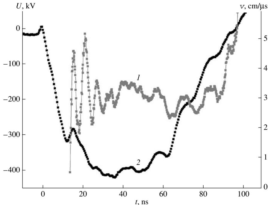
**Fig. 10.** (1) Time-dependent expansion velocity of EE plasma in a diode with a multispike cathode calculated from formula (2) at anode-cathode gaps of 11–14 mm. Curve 2 is the applied voltage.
