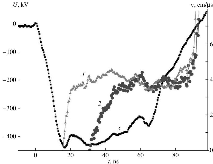
**Fig. 7.** Change in the cathode plasma expansion velocity during generation of an electron beam in a planar diode with (1) multispike and (2) solid copper cathodes. Curve 3 is the voltage.
