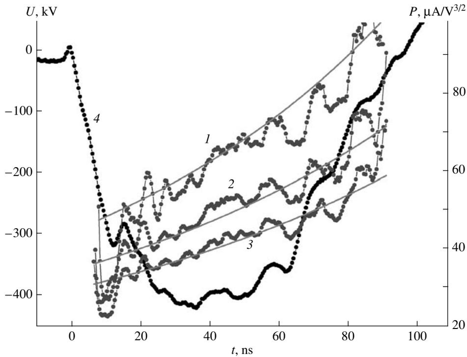
**Fig. 9.** Experimental (dots) and calculated (lines) values of the perveance of a planar diode with a multispike cathode at anode-cathode gaps of (1) 11.0, (2) 12.5, and (3) 14.0 mm. Curve 4 is the voltage.
