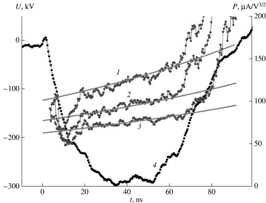
**Fig. 4.** Experimental (dots) and calculated (lines) values of the planar-diode permeance (the diode has a 60-mm-diameter carbon-fabric cathode) at gaps of (1) 10.5, (2) 12.0, and (3) 13.5 mm. Curve 4 is the voltage.
