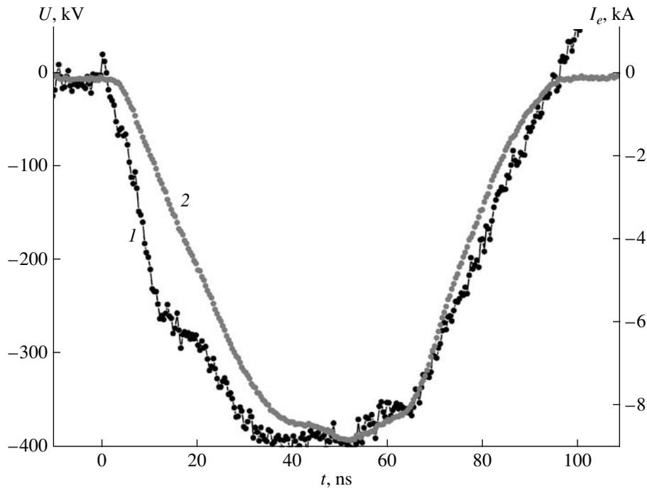
Fig. 1. Oscillograms of (1) the voltage applied to the diode and (2) the total current of the electron beam.
