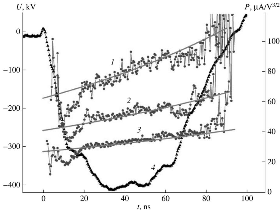
**Fig. 2.** Experimental (dots) and calculated (lines) values of the planar-diode perveance at anode–cathode gaps of (1) 9.5, (2) 12.0, and (3) 15.0 mm. Curve 4 is the voltage applied to the diode at a 15-mm gap.
