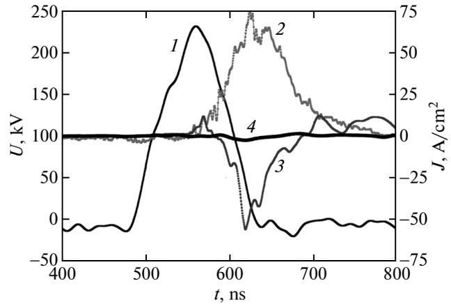
**Fig. 2.** (1) Accelerating voltage oscillogram (second pulse) and variation in the density of (2) ion and (3) compensated HPIB current. (4) Density of the current measured by the Faraday cylinder without cutoff of electrons covered by a 10- $\mu\text{m}$ -thick Al foil.
