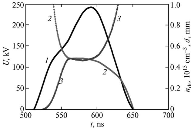
**Fig. 1.** (1) Accelerating voltage oscillogram (second pulse), (2) variation in the electron drift motion trochoid height, and (3) electron concentration in the drift region.
