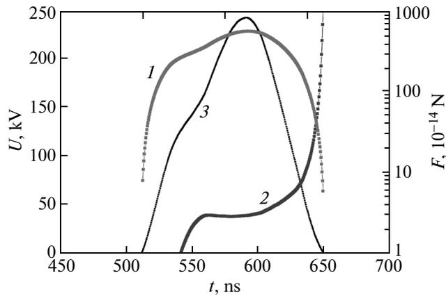
**Fig. 3.** Variation in the (1) Lorenz, Ampère, and (2) Coulomb forces acting on electrons in the drift region during ion beam generation. (3) Accelerating voltage (second pulse).
