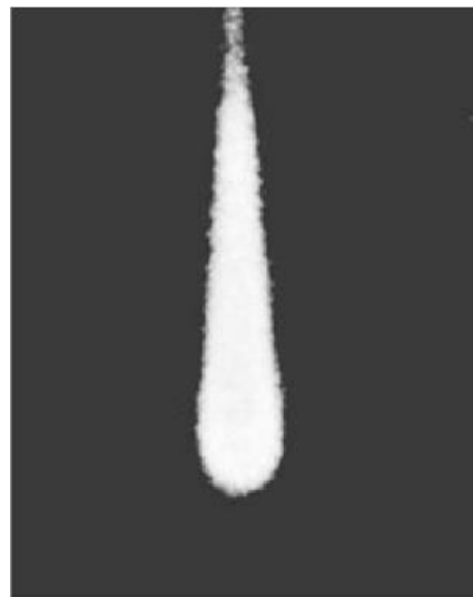
Fig. 15. Cloud chamber photograph of a single electron avalanche (from [18])
