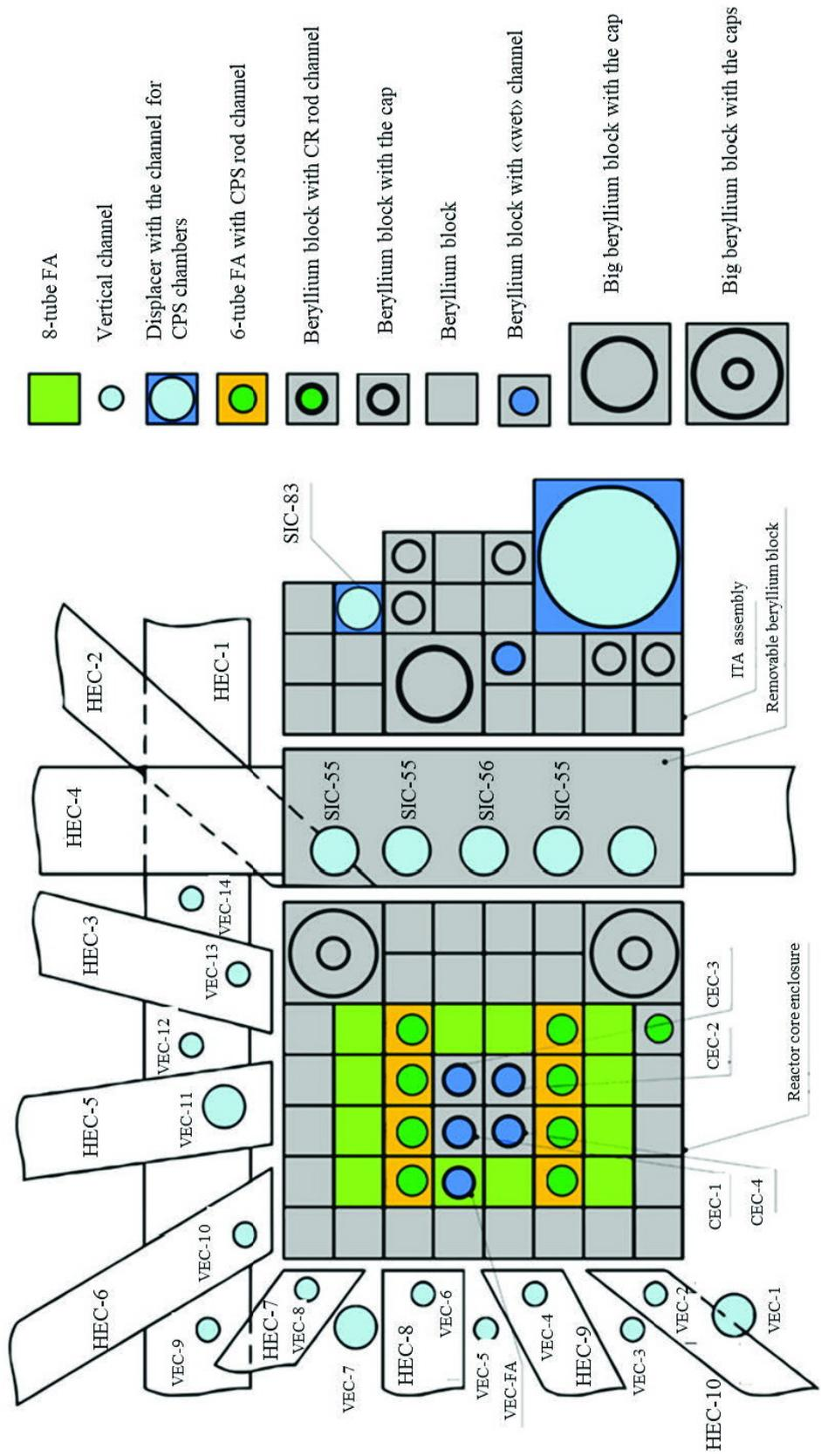
Fig. 1.2. Cartogram of the core and experimental devices of the IRT-T reactor
