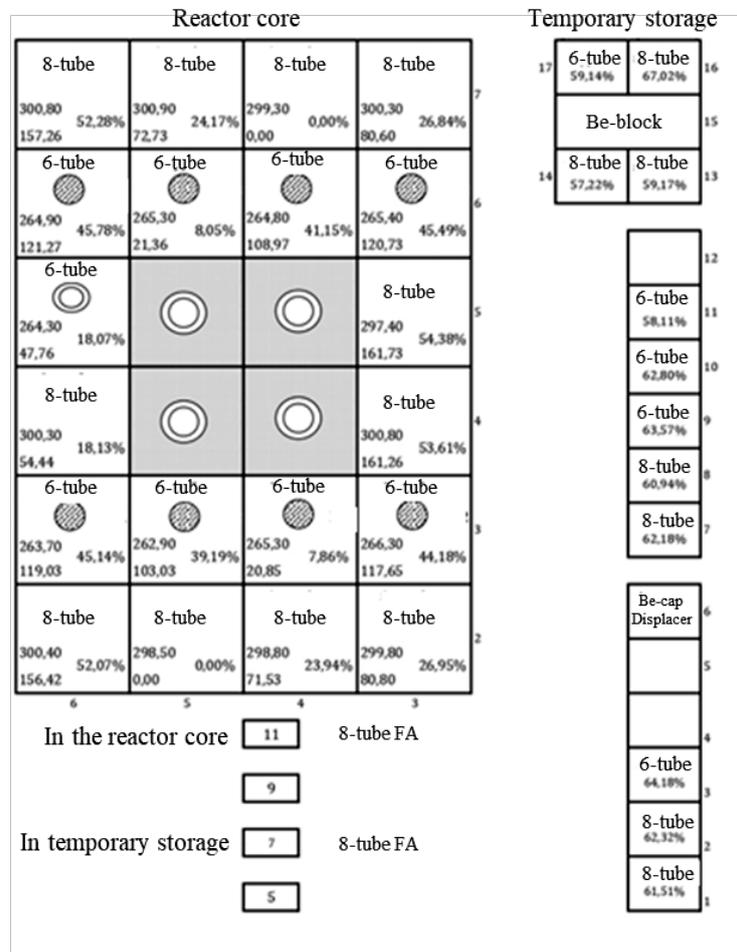
Fig. 1.5. Operating load of the IRT-T reactor
