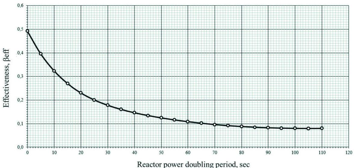
*Fig. 5.1. Dependence of CR operating rod efficiency on the doubling time of the IRT-T reactor capacity*
