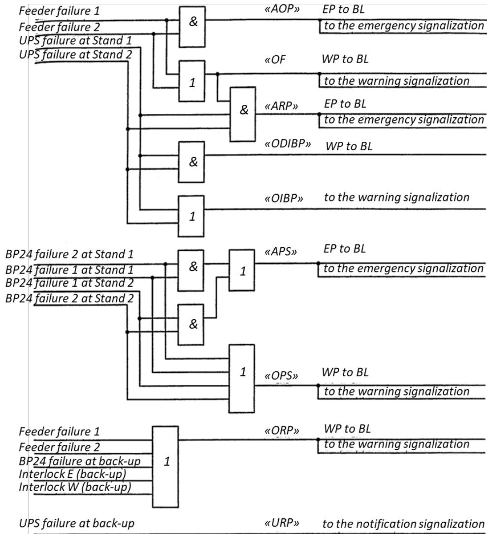
Fig. 4.5. Functional diagram of command generation for CPS power failures of the IRT-T reactor
