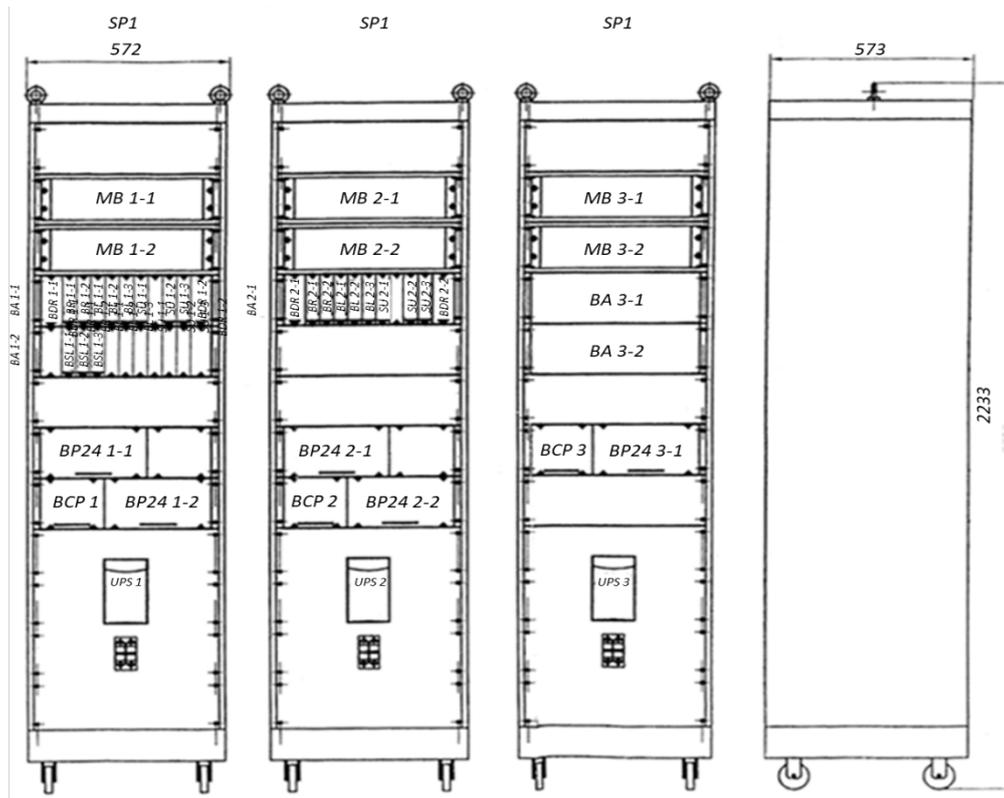
Fig. 4.1. CPS device stands of the IRT-T reactor
