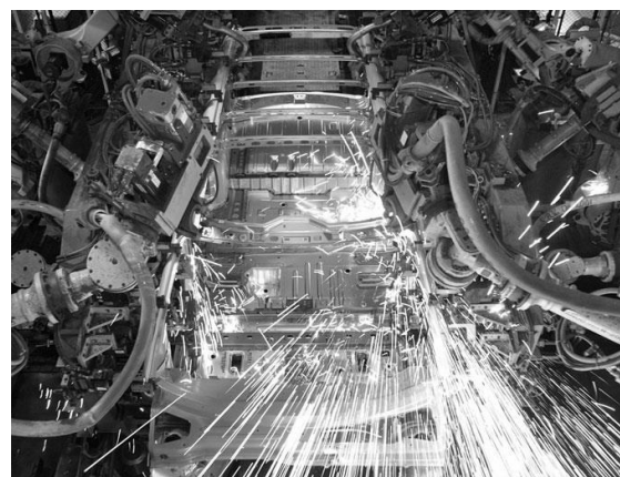
Fig. 2: Process of car frame welding
