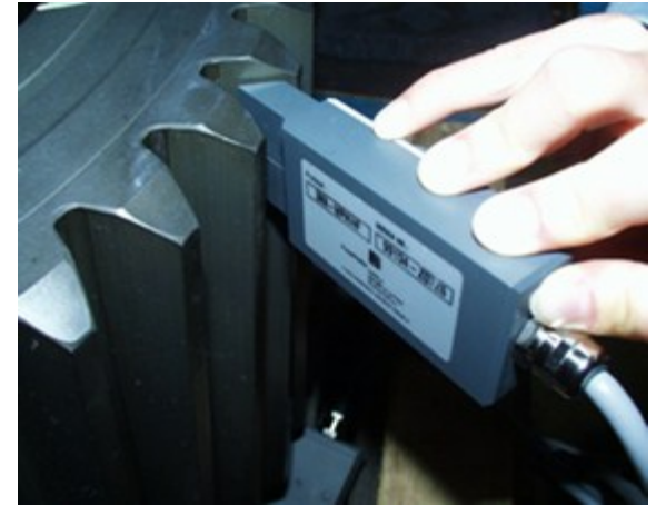
Final inspection of gear wheels after grinding
