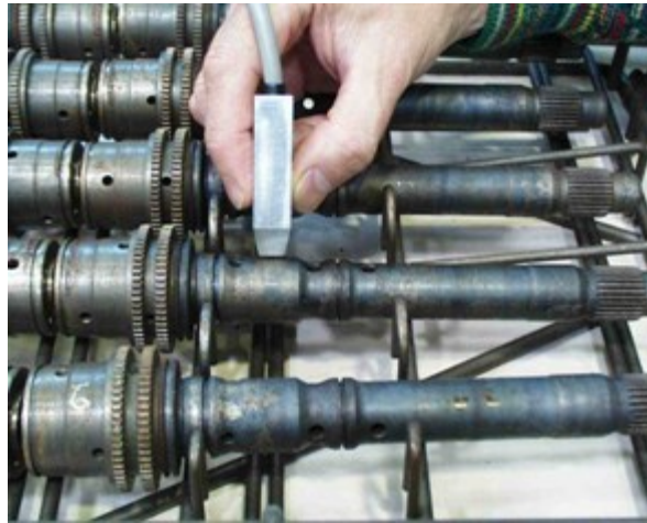
Final inspection of components after induction hardening
