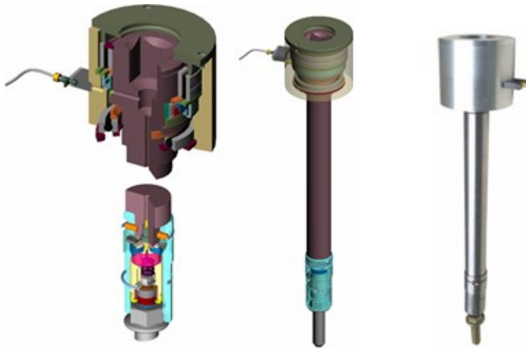
Ultrasonic sensor integrated into the screwnut of a power screwdriver
