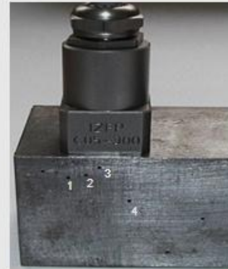
Partial View of Test Specimen with Transducer
