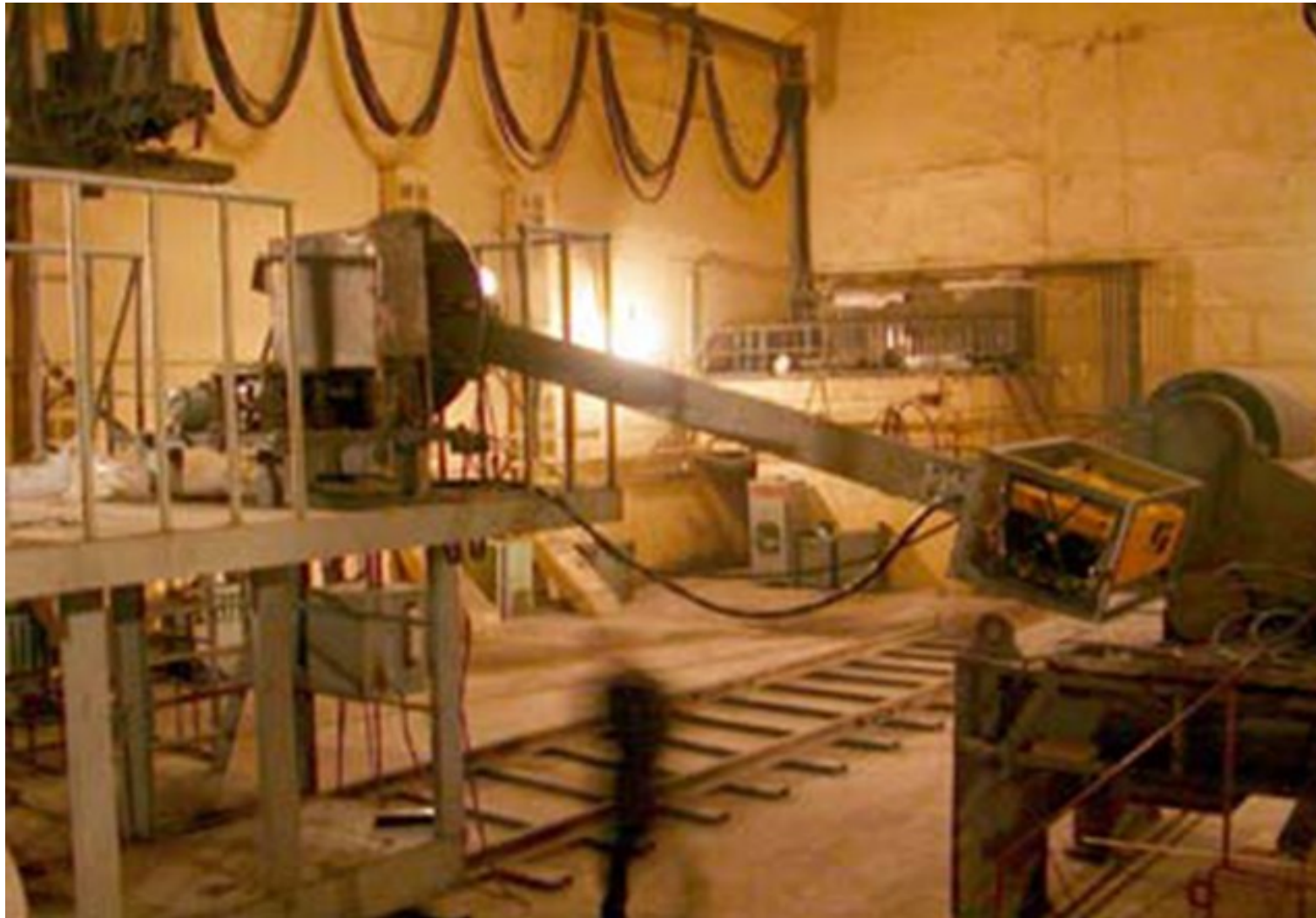
7.5 MeV Betatron Inspection Station in Volgogradneftemash production plant, Russia
